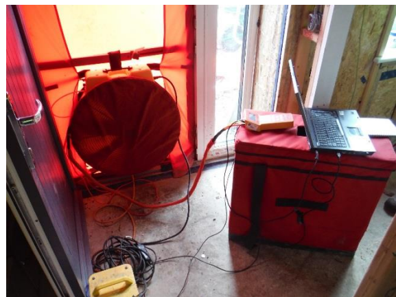
Figure 27: Air test in operation
